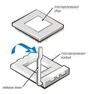
Figure 8-10. Removing the Microprocessor
